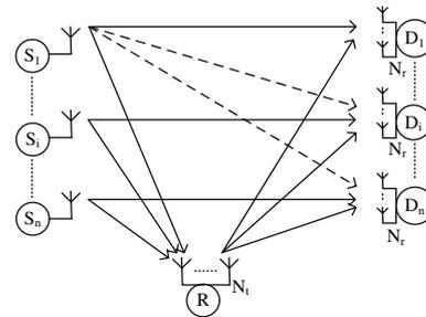
Fig. 1. Interference Relay Channel with  $n$  pairs. Only the interference from  $S_1$  are illustrated (dashed lines).
