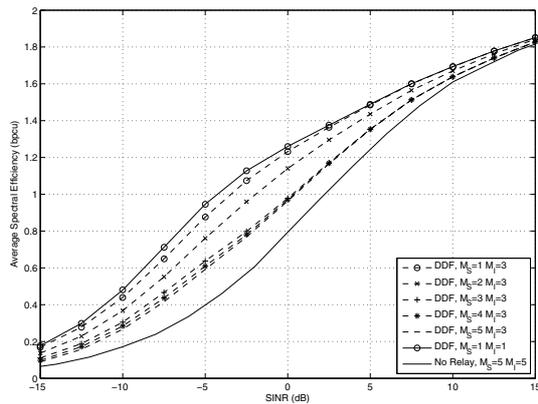
Fig. 5. Average spectral efficiency at  $D$  maximized over the available coding rates, according to the SINR,  $P_R/P_S = 6dB$ ,  $N_r = 1$  for  $(M_S, M_I) \in \{(1, 1), (5, 5)\}$  and all possible  $M_S$  for  $M_I = 3$ . The relay uses the DDF protocol with an optimized precoder.
