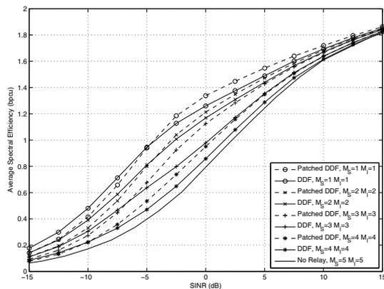
Fig. 6. Average spectral efficiency maximized over the coding rates, according to the SINR observed at  $D$ ,  $P_R/P_S = 6dB$ ,  $N_r = 1$  for  $M_S = M_I \in \{1, 2, 3, 4, 5\}$ . The relay uses the optimized precoder for the DDF protocol or the Patched DDF protocol.
