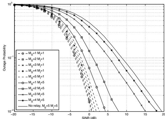
Fig. 3. Average outage probability at  $D$  according to the SINR,  $P_R/P_S = 6dB$ ,  $N_r = 1$ . The relay uses DDF protocol with optimized precoder.
