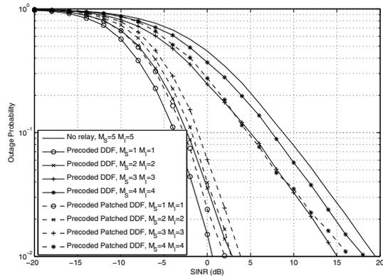
Fig. 4. Average outage probability at  $D$  according to the SINR,  $P_R/P_S = 6dB$ ,  $N_r = 1$  for  $M_S = M_I \in \{1, 2, 3, 4\}$ . The relay uses the optimized precoder for the DDF protocol or the Patched DDF protocol.
