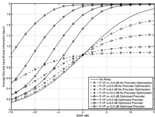
Fig. 2. Impact of the precoder optimization on the average QSPK input mutual information between the source and destination according to the SINR observed at  $D$ ,  $P_R/P_S$ , for  $n = 2$ ,  $N_r = 1$  and  $N_t = 2$ .
