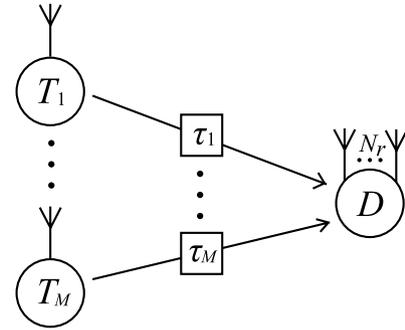
Fig. 1. Asynchronous wireless network model with  $M$  transmitters and  $N_r$  receive antennas.
