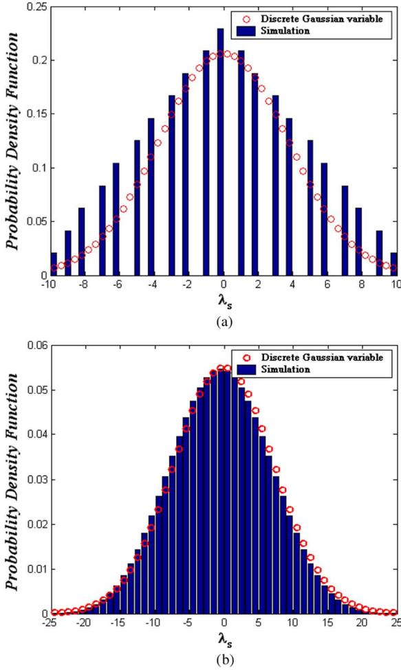
Fig. 1. PDF of the codebook induced by the sum of codewords compared to the Gaussian model. (a) Probability density function for  $N=2$ . (b) Probability density function for  $N=5$ .
