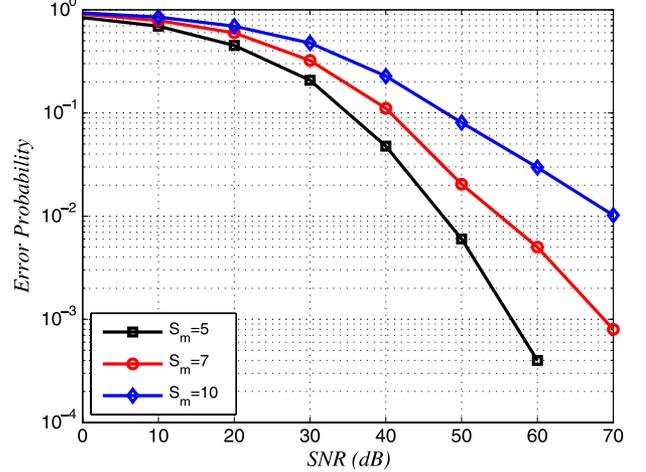
Fig. 7. Error probability using the IDA decoding.
