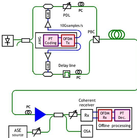
Fig. 7 PolMux OFDM experimental set-up.
