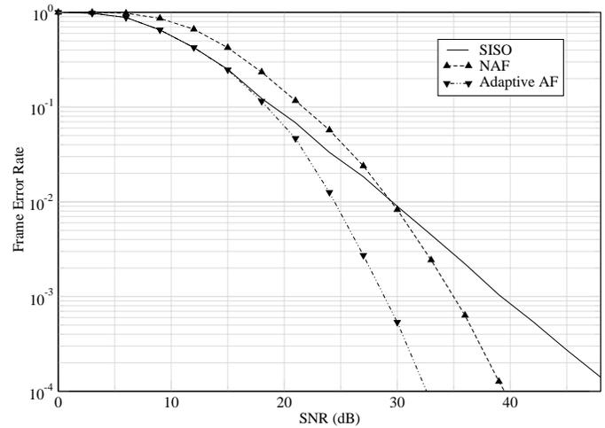
Fig. 7. 2-relays scheme: comparison of the performance of the non-cooperative case, the NAF protocol and the Adaptive AF for 4 bits pcu
