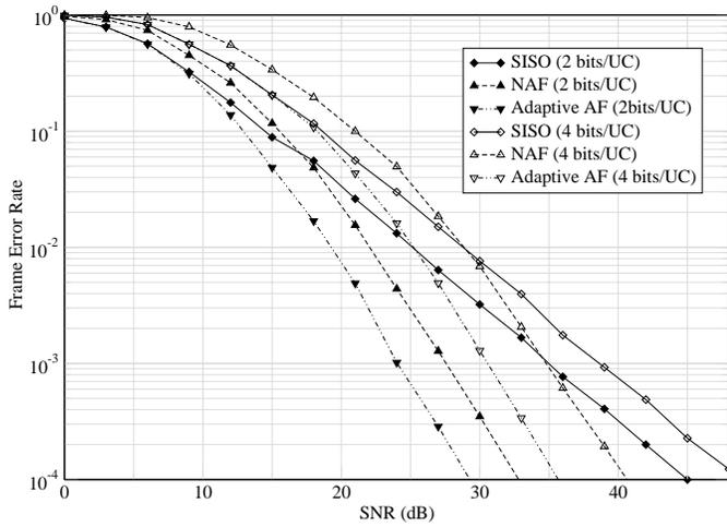
Fig. 5. 1-relay scheme: comparison of the performance of the non-cooperative case, the NAF protocol and the Adaptive AF for 2 bits pcu and 4 bits pcu
