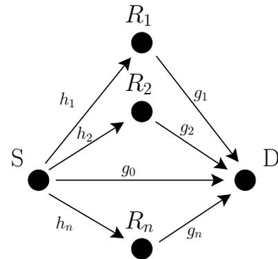
Fig. 1. System model : a relay channel with one source,  $N$  relays and one destination
