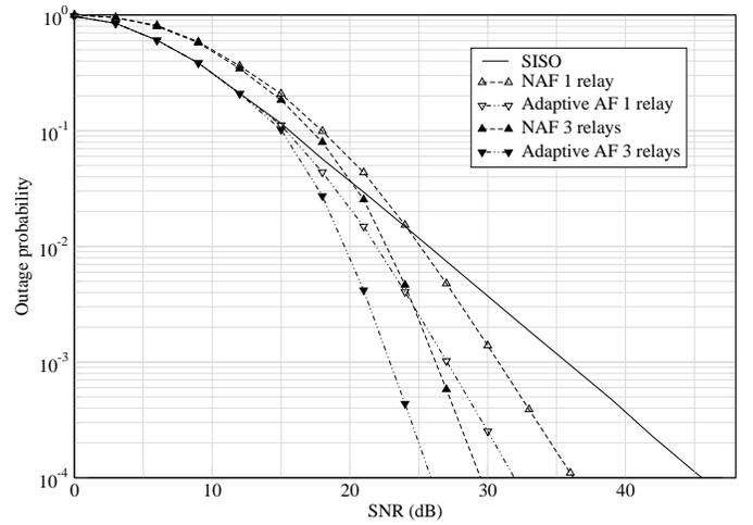
Fig. 3. 1-relay scheme: comparison of the outage probabilities of the non-cooperative case, the NAF protocol and the Adaptive AF for 4 bits pcu
