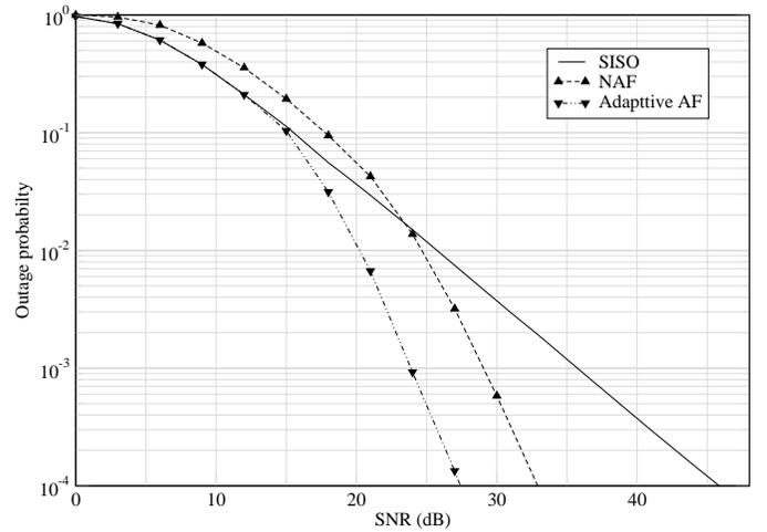
Fig. 4. 2-relays scheme: comparison of the outage probabilities of the non-cooperative case, the NAF protocol and the Adaptive AF for 4 bits pcu
