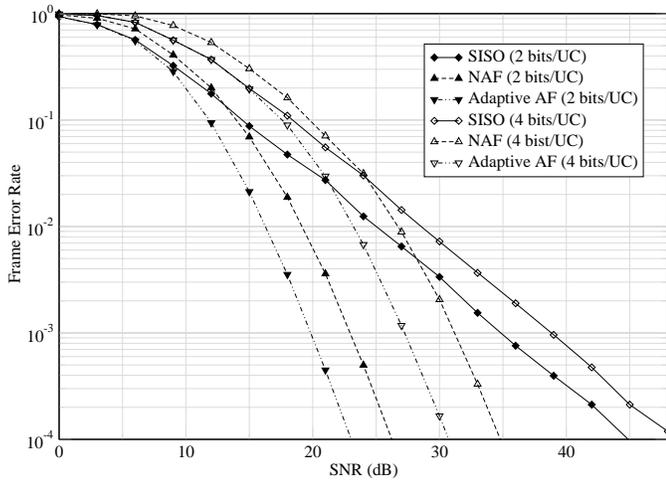
Fig. 6. 1-relay scheme: comparison of the performance of the non-cooperative case, the NAF protocol and the Adaptive AF for for 2 bits and 4 bits pcu, with 1 relay chosen out of 3
