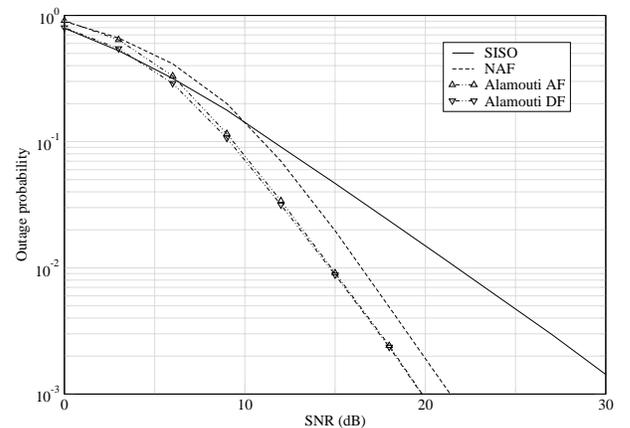
Fig. 2. Comparison of the outage probabilities of the SISO, NAF and Alamouti AF and DF protocols for 2 bits spectral efficiency
