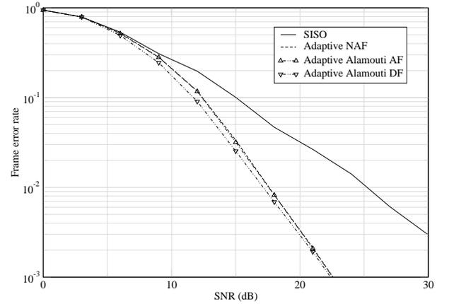
Fig. 6. Comparison of the performance of the non-cooperative case, the Adaptive NAF and the Adaptive Alamouti AF and DF for 2 bits spectral efficiency
