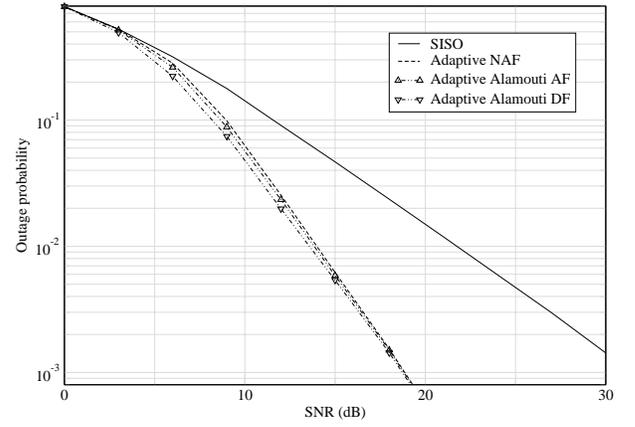
Fig. 5. Comparison of the outage probabilities of the non-cooperative case, the Adaptive NAF and the Adaptive Alamouti AF and DF for 2 bits spectral efficiency
