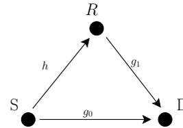
Fig. 1. Channel model: one source, one relay, one destination
