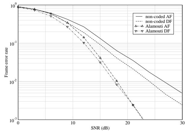
Fig. 8. Comparison of the performance of the non-coded AF, non-coded DF and Alamouti DF for 4 bits spectral efficiency
