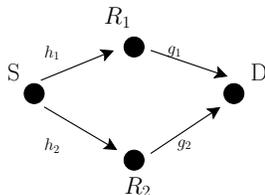
Fig. 7. Channel model: one source, two relays, one destination
